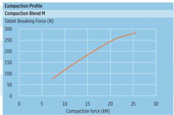
Tablet press: IMA Styl'One 105ML, Tablets: Ø 11.3 mm, 500 mg
